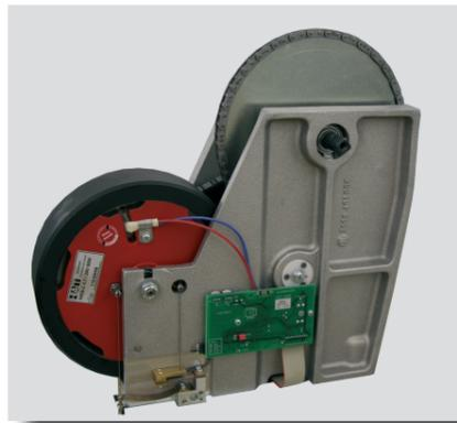
The actual "drive and brake unit" is housed in a special aluminum die-cast enclosure. In contrast to the simple sheet metal fixtures used in many home ergometers, our design ensures smooth running and reliable mounting of axles and bearings. With the electronically controlled eddy-current brake the set load in watts is precisely maintained.
