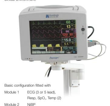
Users can upgrade their monitors at any time by simply adding a module to their existing configuration to further extend the units capability.
